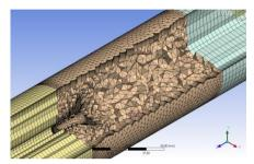
Inlet section to the left and outlet section to the right meshed using sweeping method, as central part using patch-independent tetrahedral method. Every solid wall have inflation layer of 10 prismatic elements to accurately resolve shape of boundary layer near the wall. Overall mesh quality is suitable for CFD simulation, and coarse indeed to meet system requirements of personal computer.
