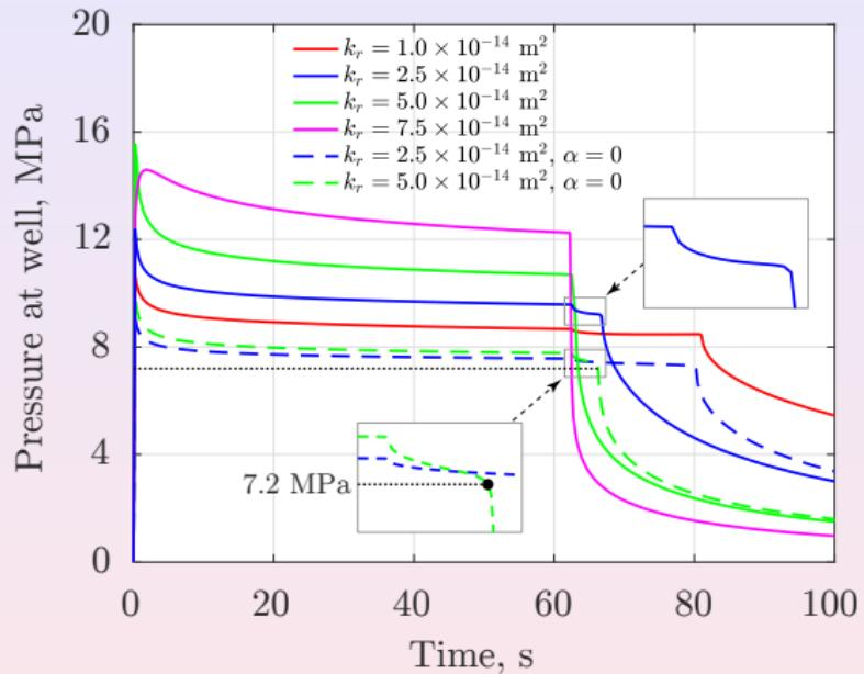
**Pressure at wellbore** for different permeability values in coupled ( $\alpha = 0.75$ ) and uncoupled ( $\alpha = 0$ ) cases
