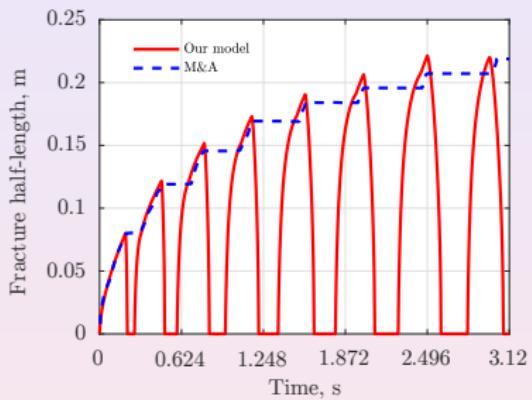
Time histories of fracture **width at wellbore** and fracture **half-length** in case of multiple injections  $Q_{multiple}(t)$
