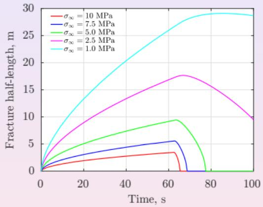
Fracture **half-width at wellbore** and **half-length** for different closure stress values
