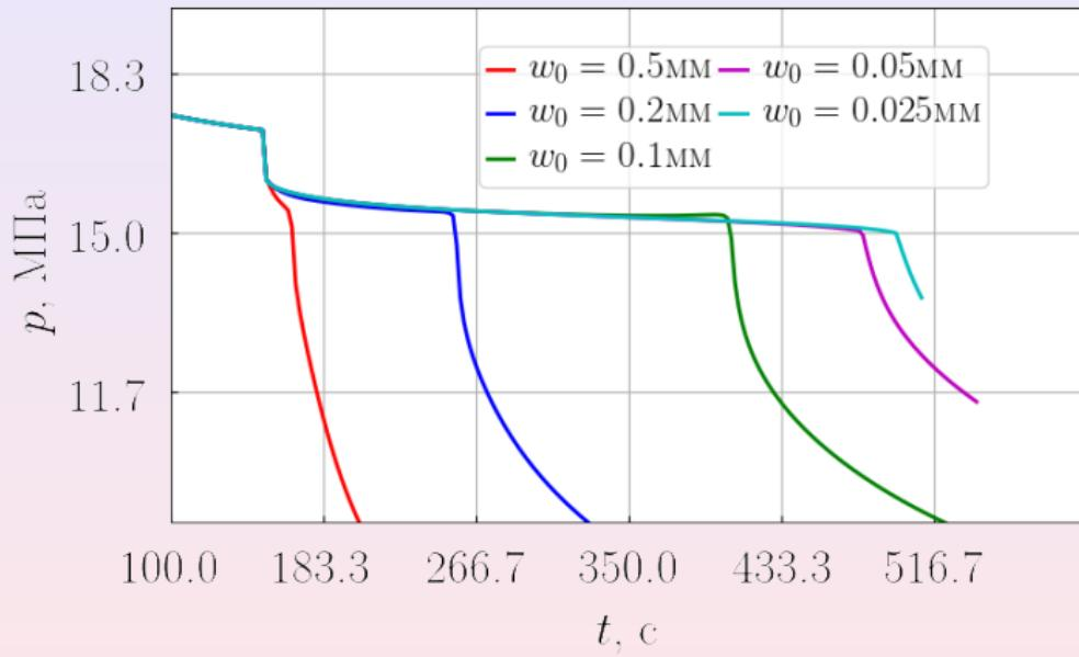
Sensitivity analysis of the PDC to residual half-aperture
