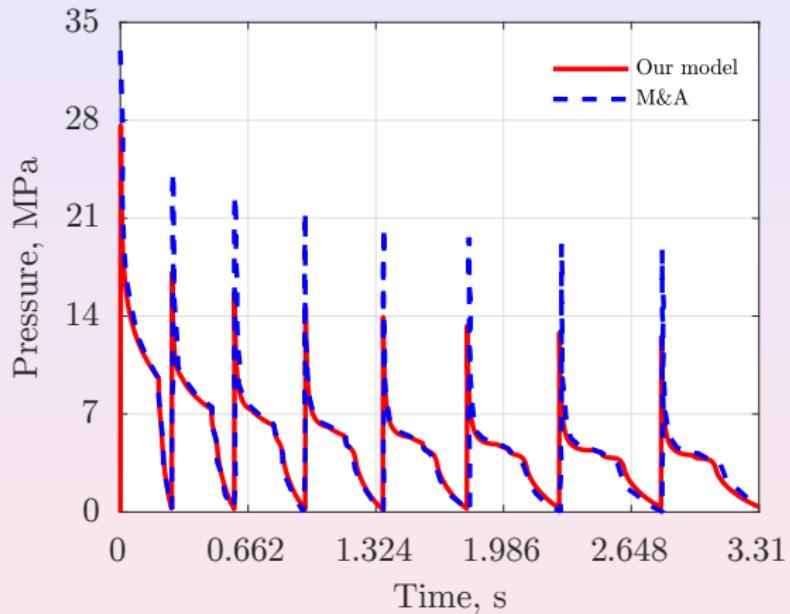
Pressure at wellbore in case of multiple injections  $Q_{multiple}$
