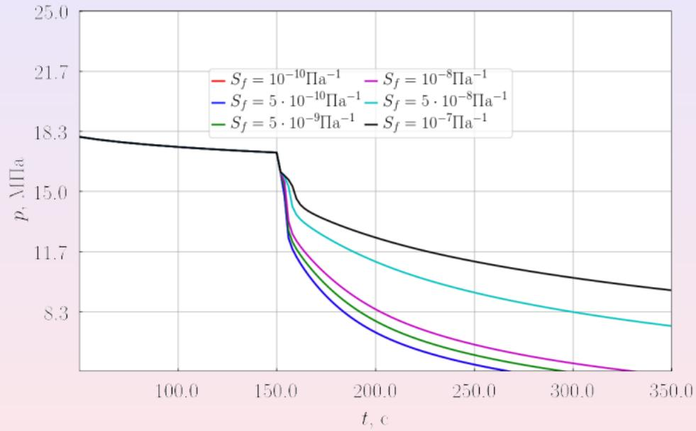
Sensitivity analysis of the PDC to fracture **stiffness** ( $w_0 = 0.2 \text{ mm}$ )
