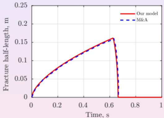
Time histories of fracture **width at wellbore** and fracture **half-length**
