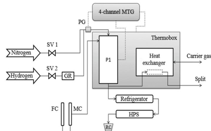
**Fig. 2.** Technological diagram of a laboratory catalytic installation
