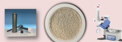
The resulting composites ZSM-5:ZSM-12, ZSM-5:MCM-41 were mixed with bohemite in 60:40 % wt. ratio and extruded, then Pt was deposited over the extrudates by incipient wetness impregnation method in the amount of 0.5 % wt.
